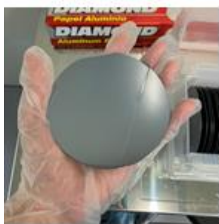
4-inch wafer silicon wafer
