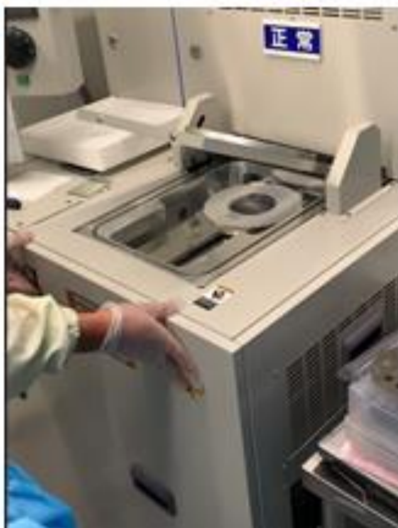
Advanced Silicon Etcher Si reactive ion etching (RIE) Etching
