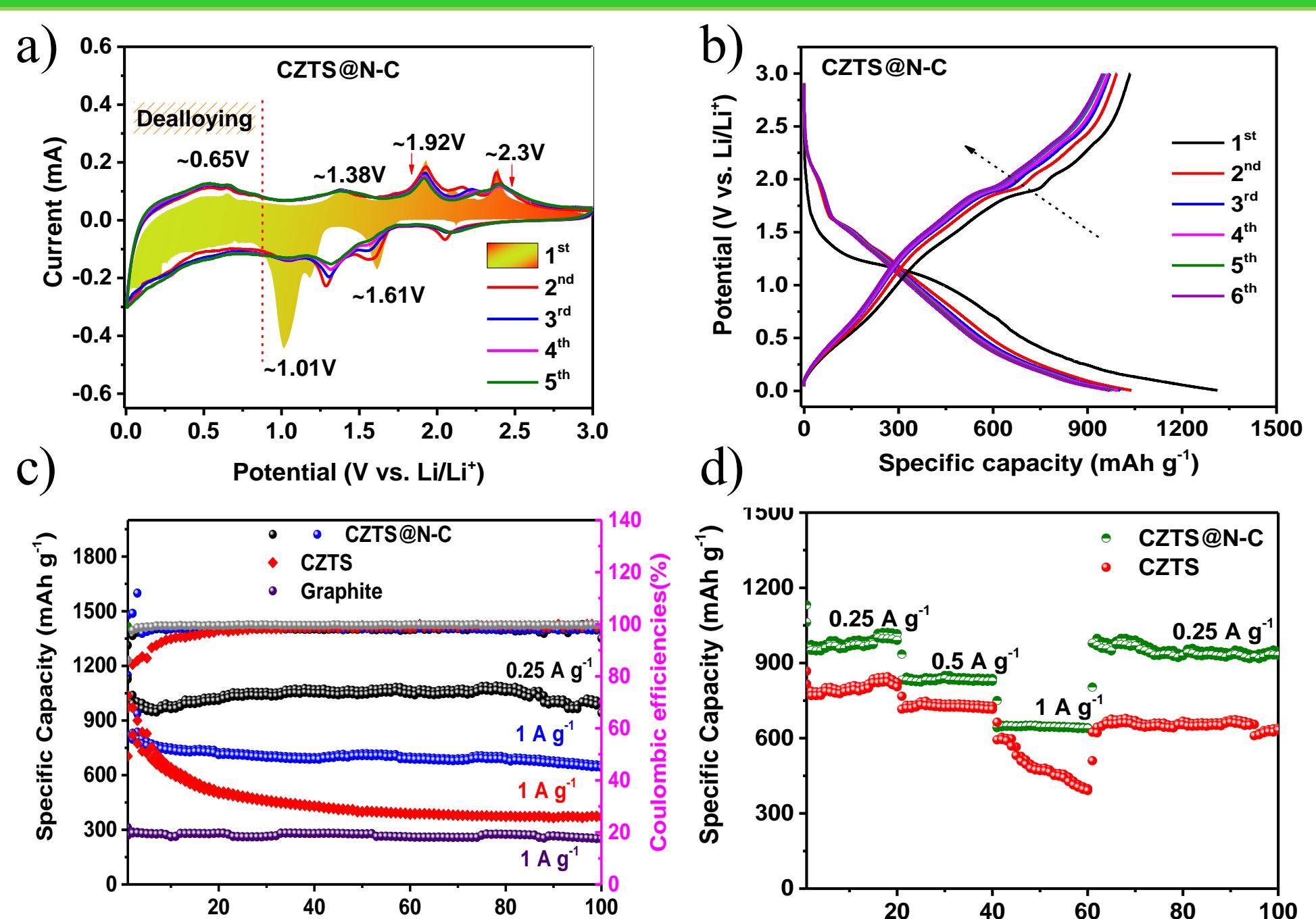
(a) CV curves of CZTS@N-C with 0.1 mV/s scan rate and (b) charge-discharge curves of CZTS@N-C at a rate of 1 A/g. (c-d) Electrochemical performance of CZTS, CZTS@N-C and graphite anode materials.
