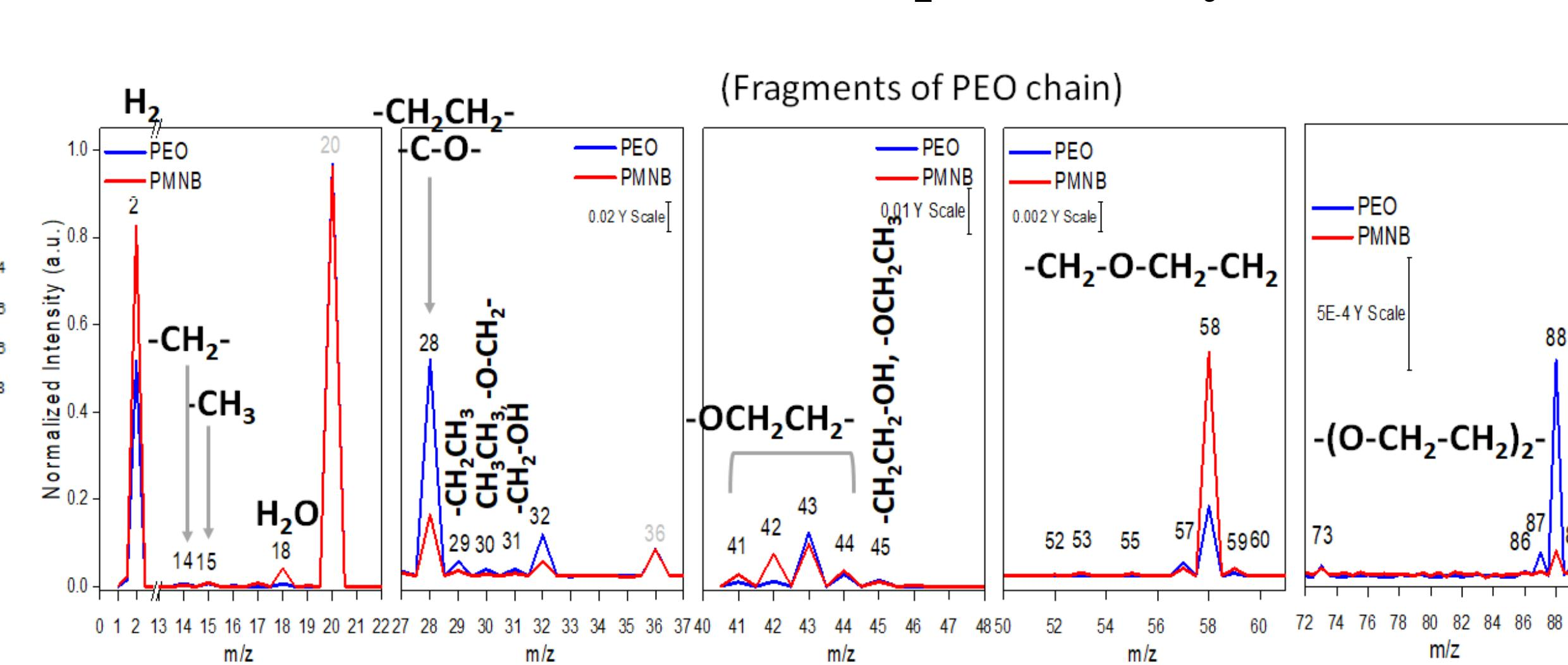
Less gas evolution is obtained with PMNBs polymer electrolyte. PEO will be decomposed during cycling.
