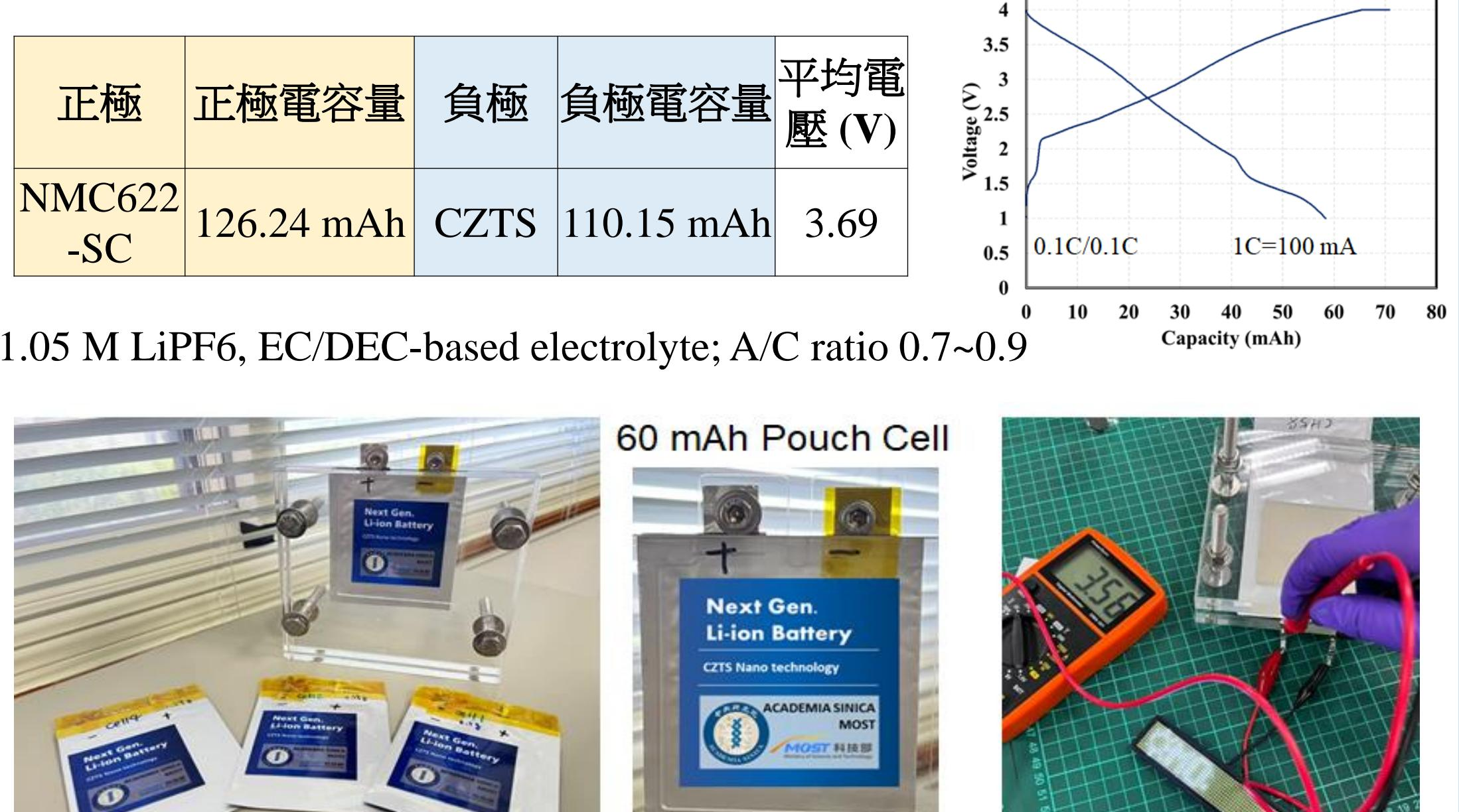
A full cell (NCM622/CZTS) with 60 mAh is obtained in the pouch cell (57mm × 61 mm size).
