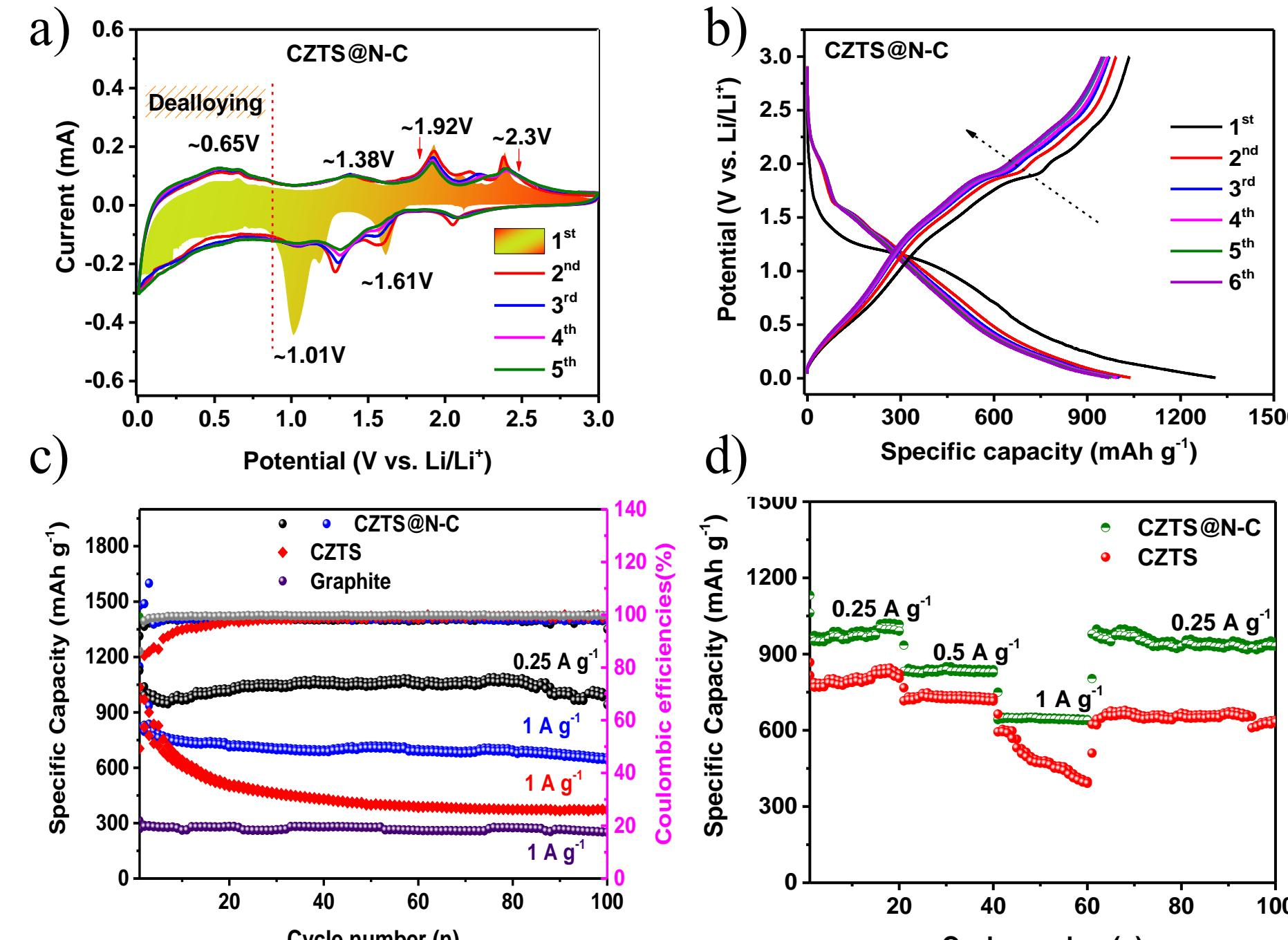
(a) CV curves of CZTS@N-C with 0.1 mV/s scan rate and (b) charge-discharge curves of CZTS@N-C at a rate of 1 A/g. (c-d) Electrochemical performance of CZTS, CZTS@N-C and graphite anode materials.
