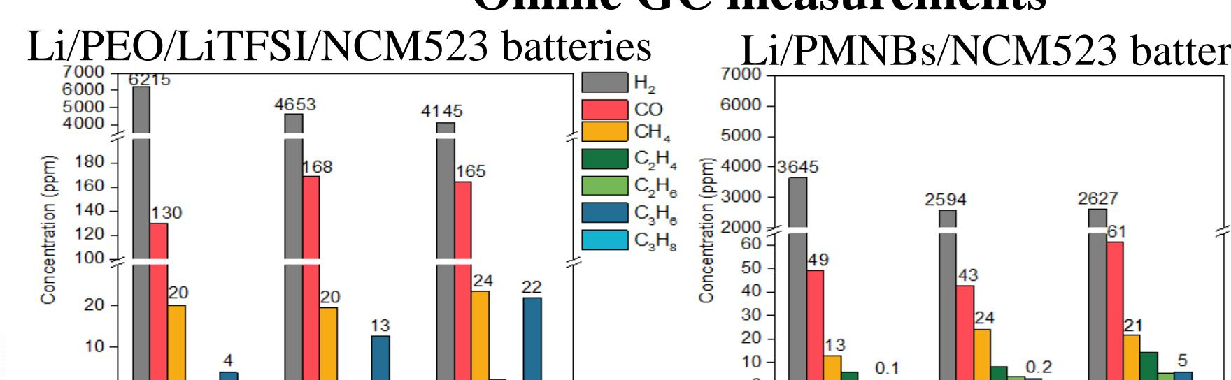
Less gas evolution is obtained with PMNBs polymer electrolyte. PEO will be decomposed during cycling.
