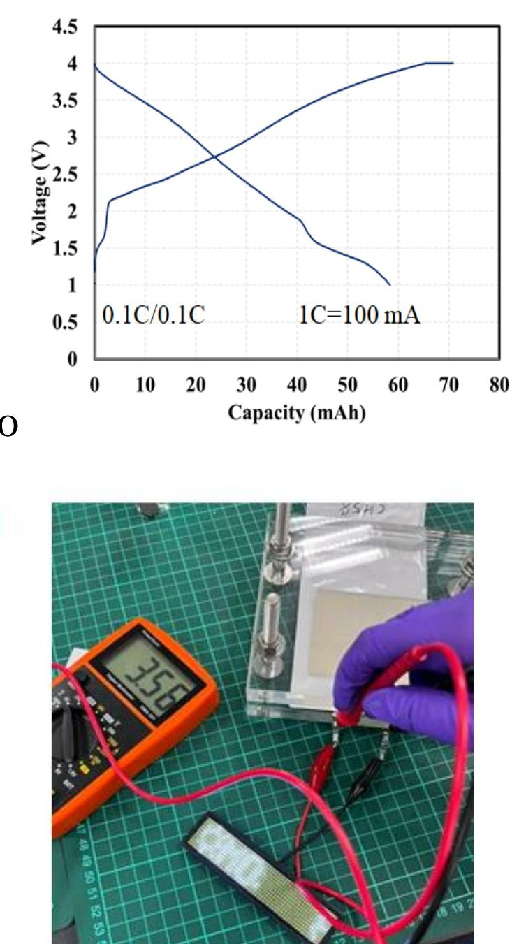
A full cell (NCM622/CZTS) with 60 mAh is obtained in the pouch cell (57mm x 61 mm size).
