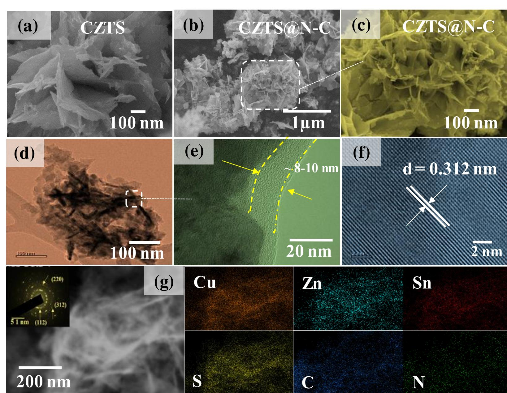
SEM image of (a) pristine CZTS and (b-c) CZTS@N-C composites (d) TEM image of CZTS@N-C, (e-f) The HRTEM images of CZTS@N-C composites. (g) The STEM-EDX elemental mapping of CZTS@N-C including dark-field images, Cu, Zn, Sn, S, C and N maps.
